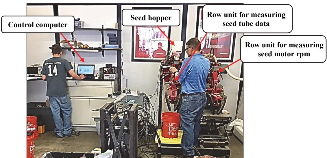
**Figure 1.** The laboratory set up at the Planting Systems Laboratory where the simulated planting tests were performed.
